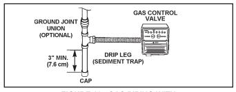
FIGURE 12. GAS PIPING WITH FLEXIBLE CONNECTOR.
